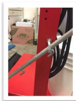
13. Use the black Velcro vinyl bag to cover the head assembly in between coats to protect the manifold and pad from drying out.
