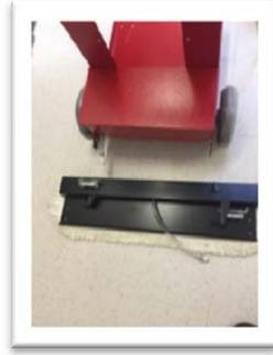
2. Insert the stud pin first, then spring latch bracket on the other side.
