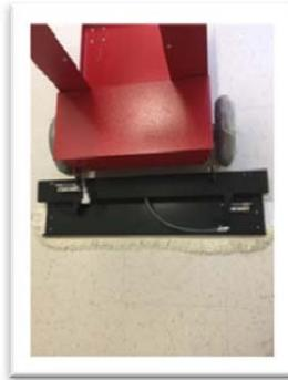
3. Attach the male plastic connector from the head assembly to the female plastic solution connector at the front of the Ultra-Trak base unit.
